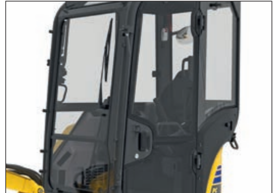
Newly designed MR-5 cabin with wider entrance, much more space for the operator and many improved safety features.
