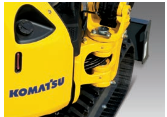
The swing cylinder is now relocated to the left side of the excavator to minimise protrusion. The operator doesn't have to worry about it when working near a wall.
